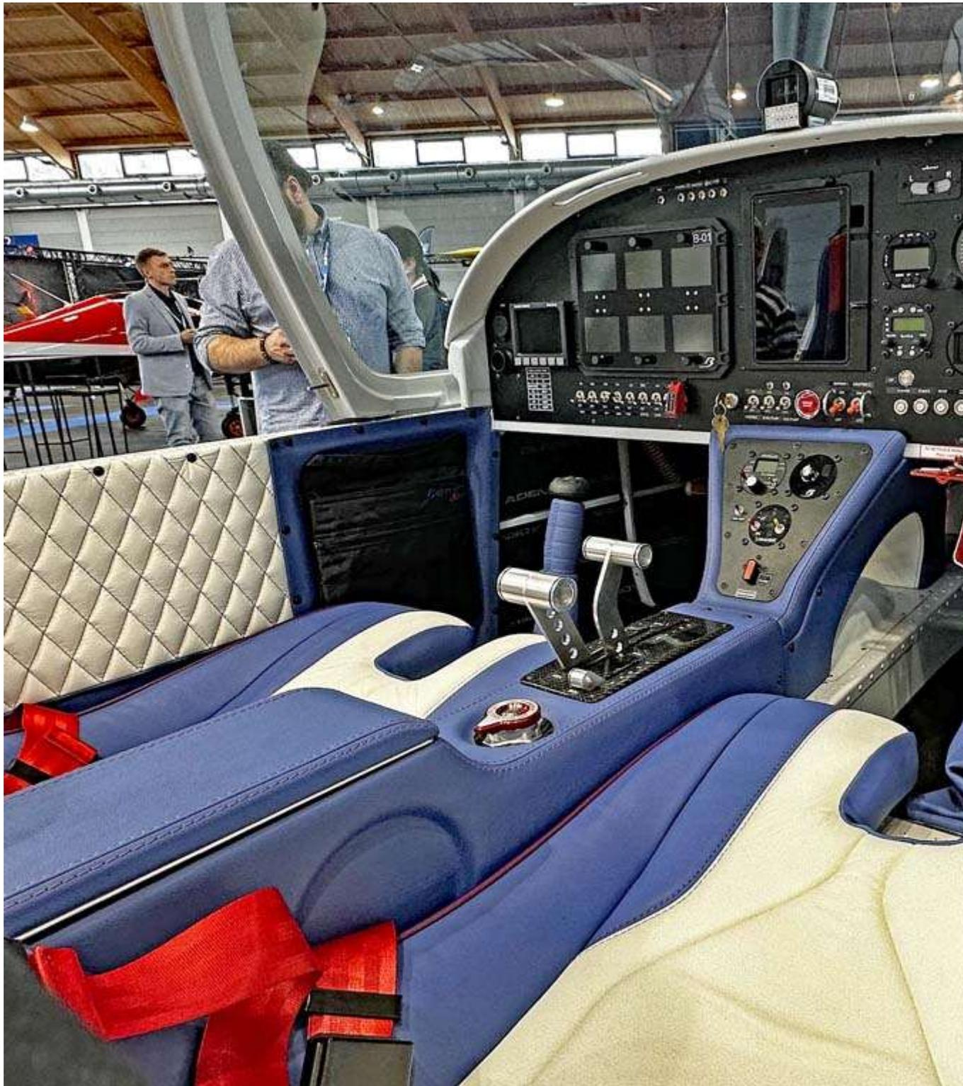
[Dan Johnson] Beautifully upholstered seats have a composite sandwich structure. Four-point seat belts are standard. Headphone jacks are located behind the pilot's seats.
